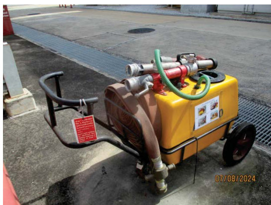
Wheel Foam Chemical Extinguisher
